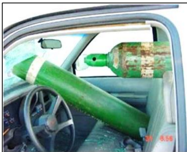
Figure 3. Unsecured cylinders when transporting the gas.
