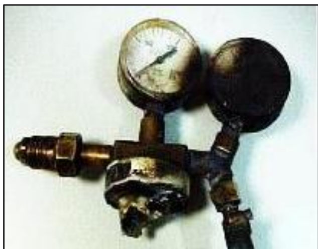
Figure 8. Oxygen explosion causing damage to the regulator and pressure gauges.
