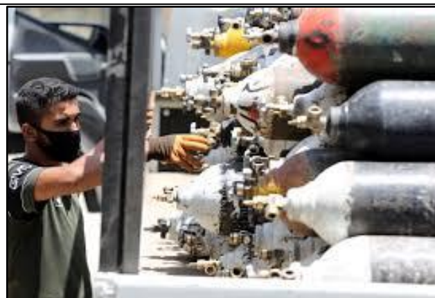
Figure 5. A very dangerous situation when storing or transporting gas cylinders.
