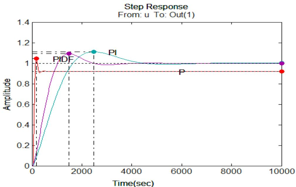
Fig. (11) Comparison between P,PI, PIDF Control response to step input.
