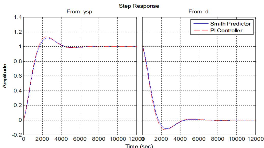
Fig. (11b) Control response to step input comparison between PI- Control and Smith predictor.
