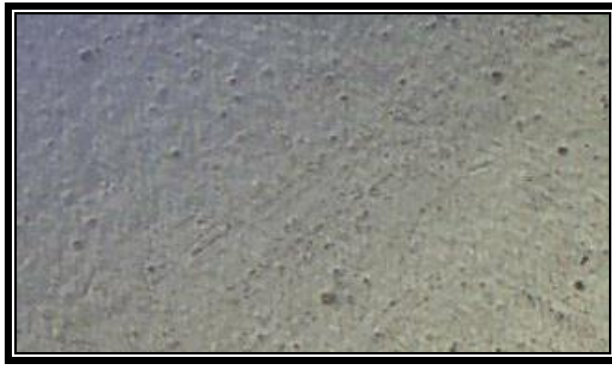
Fig.(3) Optical micrograph of (UPE/NR) polymer blend before immersion(15X).
